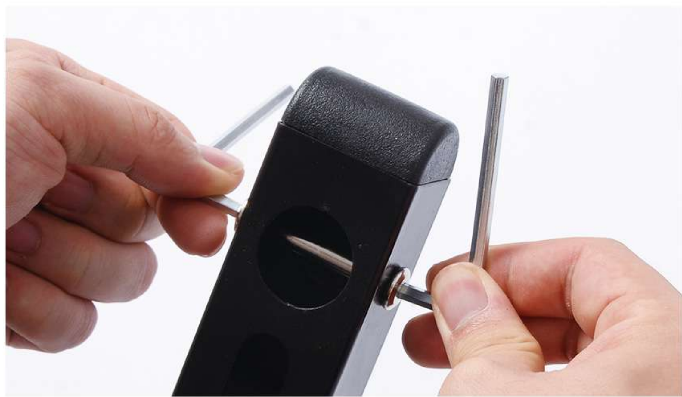
13. Use two small hex wrenches to unscrew the knob screw from the handrail.
