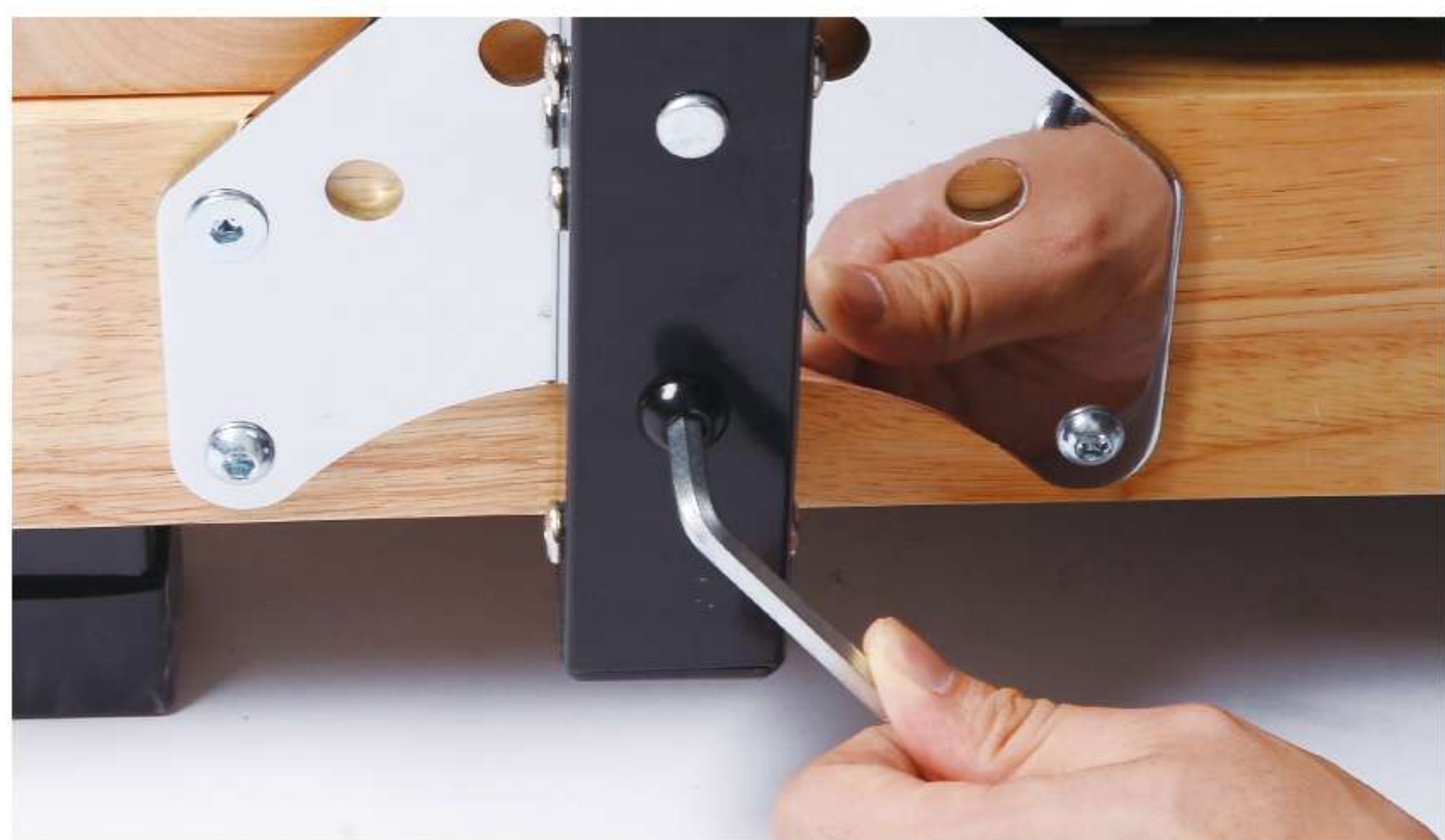
9. Use a large hex wrench to tighten the bolt.
