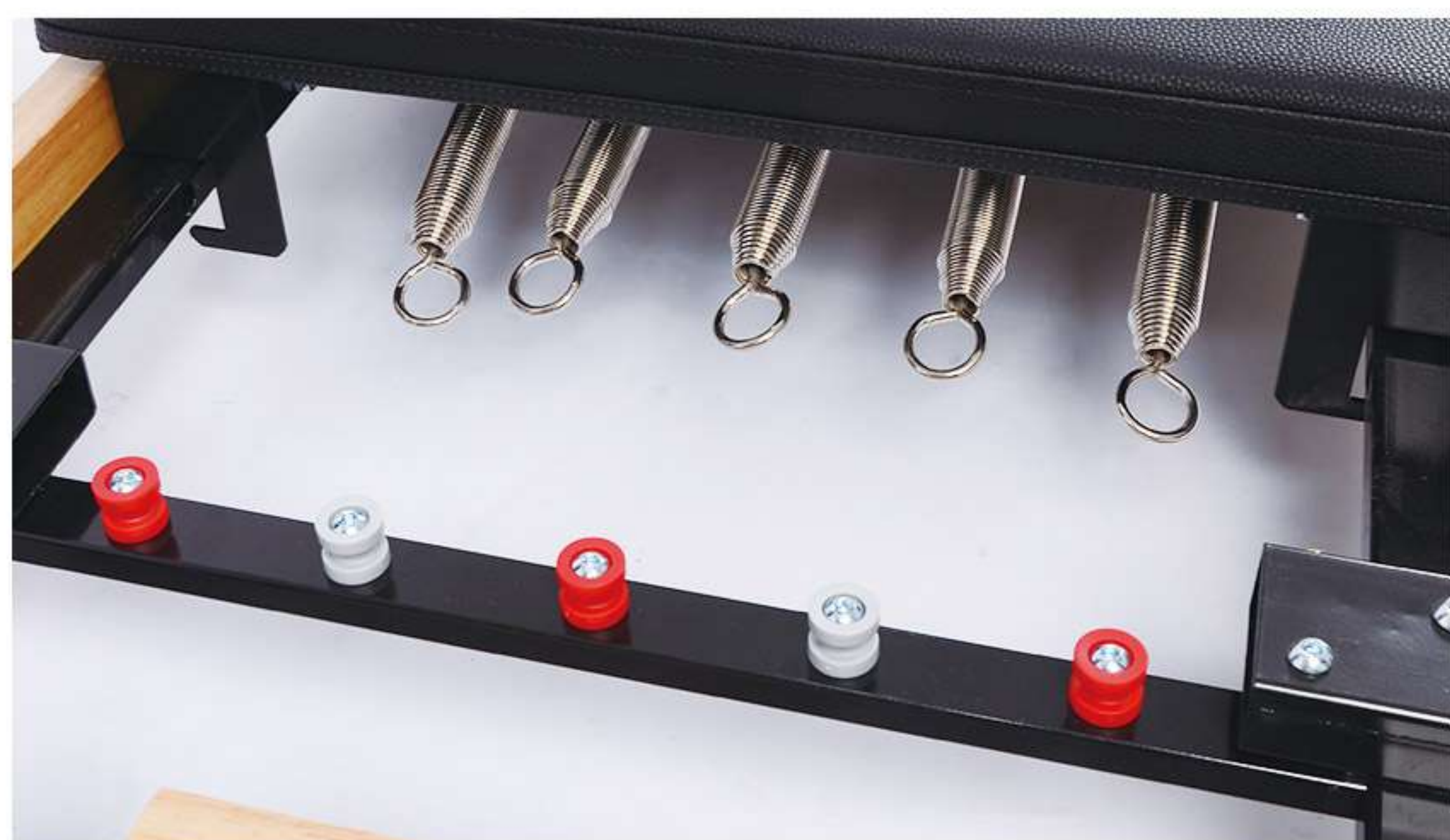
19. After removing all the springs, push the cushion back to othe side.
