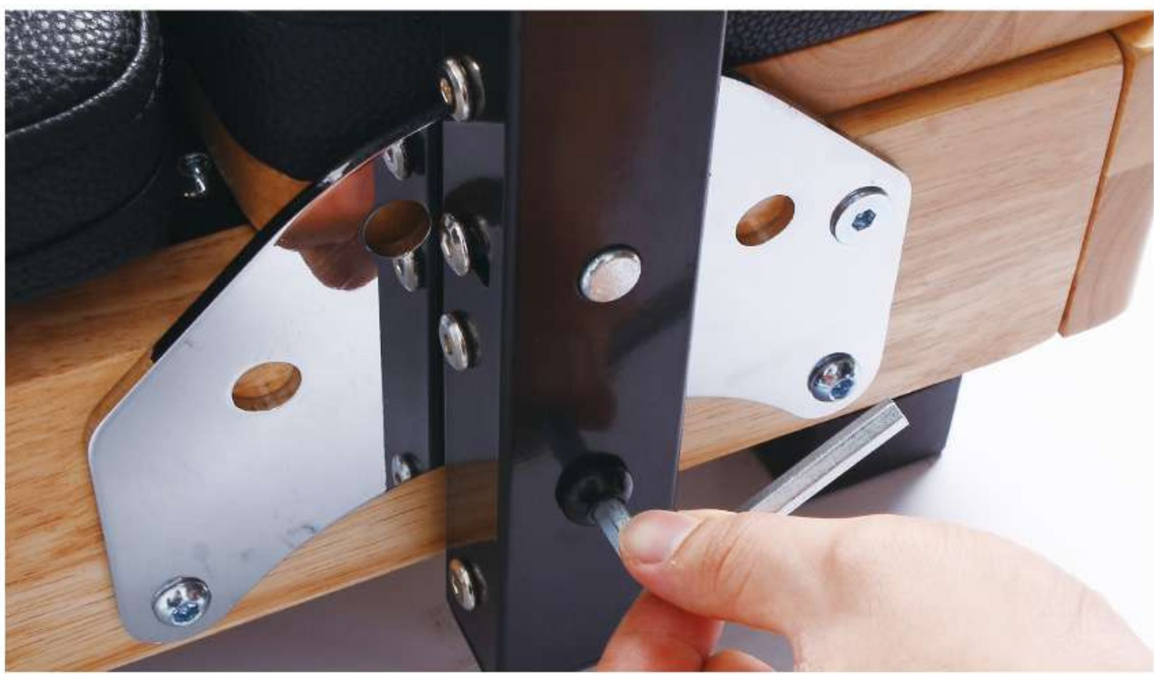
16. Insert the M10x40 screw into the spacer, insert it into the bottom hole of the armrest board, install a gasket on the other side, and tighten it with a large hex wrench.
